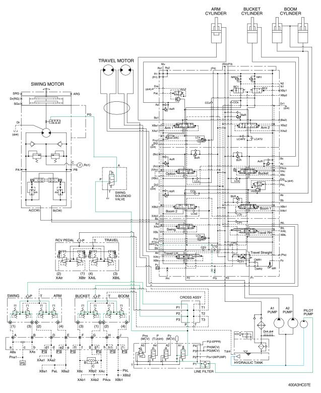
When any of the swing, arm in, boom up or travel lever is tilted, the swing brake solenoid value is shifted to the downward by the MCU that senses the pilot pressure of the RCV control lever.
