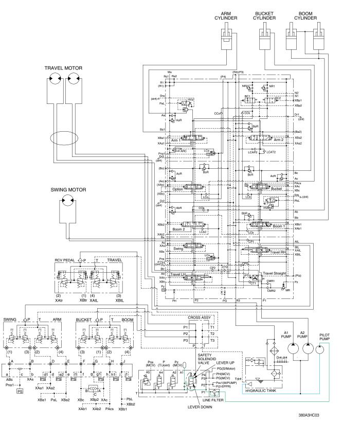
When the lever of the safety solenoid valve is moved upward, oil flows into the remote control valve through solenoid valve and line filter and cross assy.
