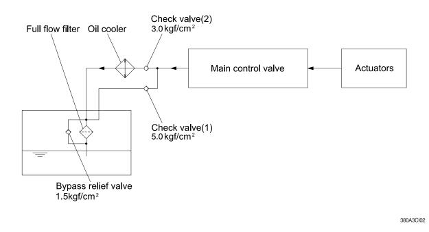
All oil from each actuator returns to the hydraulic tank through the control valve.
