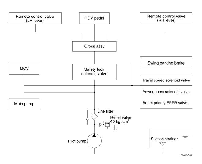
The pilot circuit consists of suction circuit, delivery circuit and return circuit.
