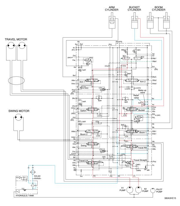
When the RH control lever is pushed right, the bucket spool in the main control valve is moved to the roll out position by the pilot oil pressure (XAc) from the remote control valve.
