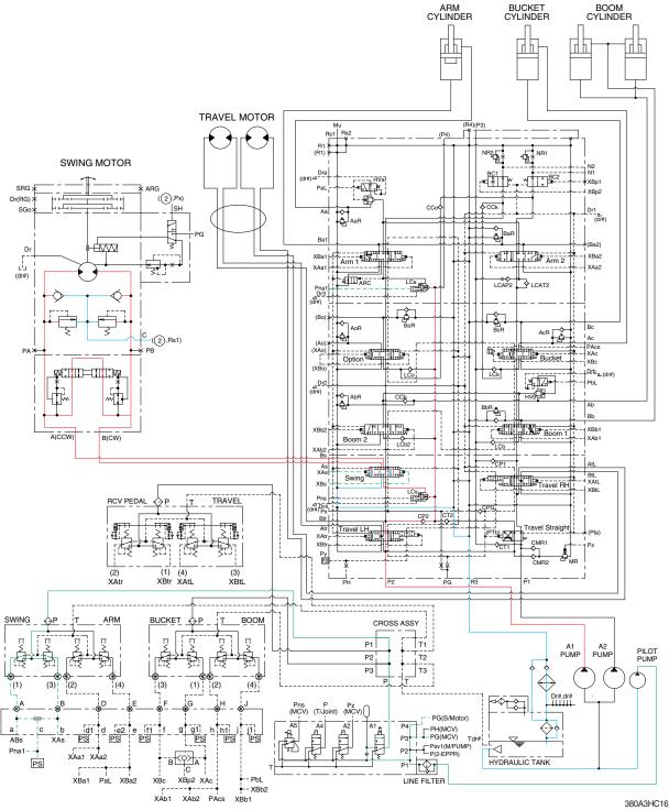
When the LH control lever is pushed left or right, the swing spool in the main control valve is moved to the left or right swing position by the pilot oil pressure (XAs, XBs) from the remote control valve. The oil from the A1 pump flows into the main control valve and then goes to the swing motor.
