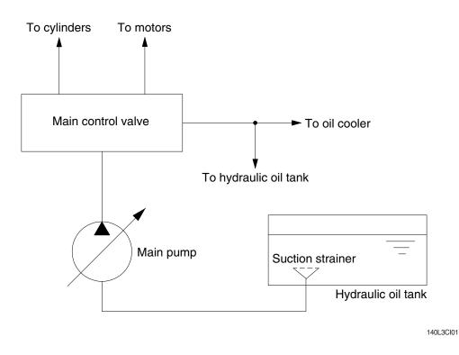
The pumps receive oil from the hydraulic tank through a suction strainer. The discharged oil from the pump flows into the control valve and goes out the tank ports.
